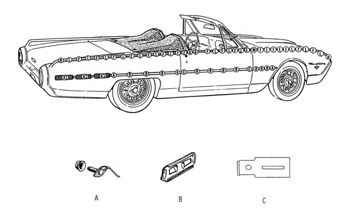
It is recommended that you mark the side of your car with a chalk line. You should key off of the center of the rear 1/4 panel bars on a 1962, and on a 1961 key off of the center between the second and third spear on the 1/4 panel. You will need a drill and drill bits to drill the holes for the clips.
